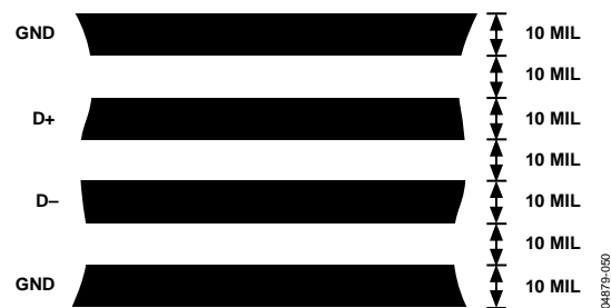
Figure 50. Arrangement of Signal Tracks
